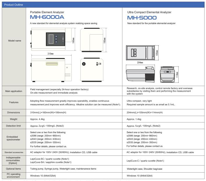
(Note1) Quartz is available only for neutral and acidic solution, and sapphire is available for neutral, acidic and alkaline solution.
